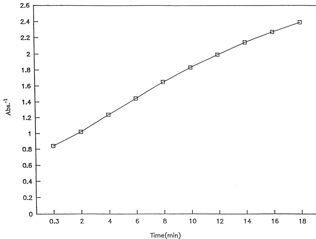
Fig. 7. Photosensitized reactions of neutral red with preirradiated cyclopentanone under anaerobic conditions.
