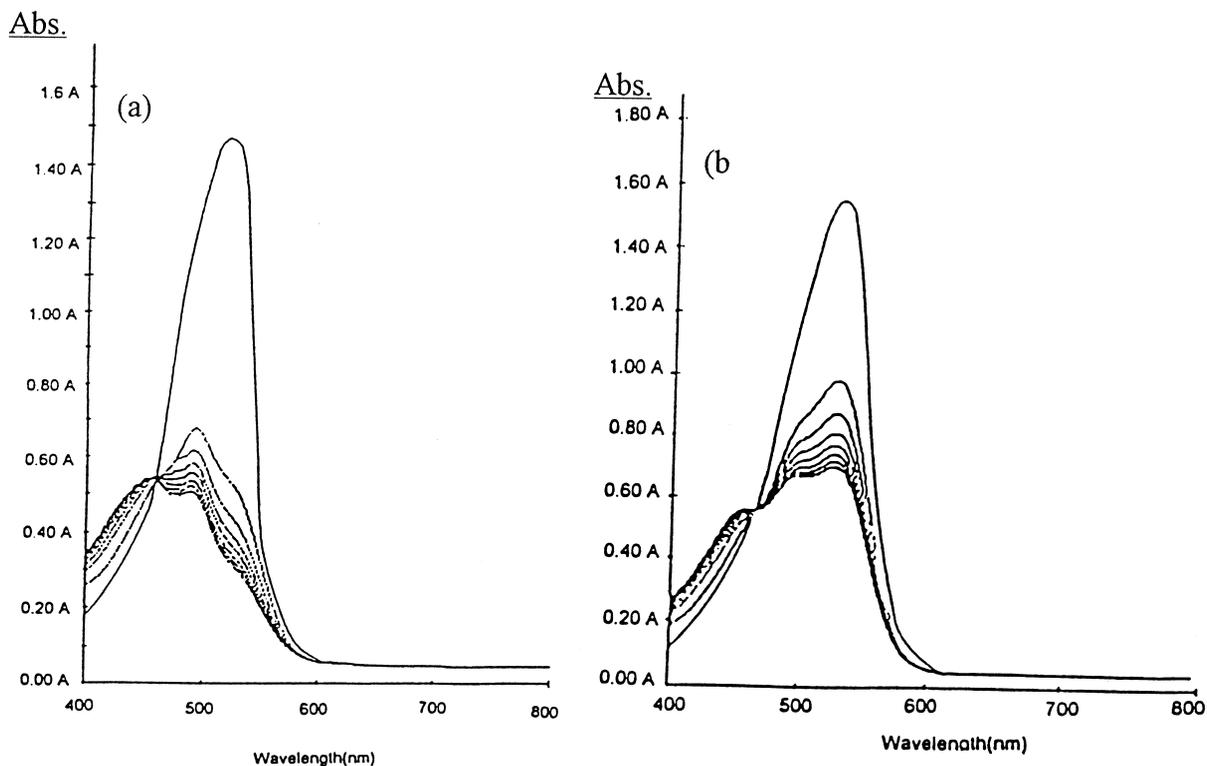
Fig. 2. Photosensitised reactions of neutral red, under anaerobic conditions, 4 min after irradiation with VIS radiation. (a) in cyclohexanone (b) in cyclopentanone.
