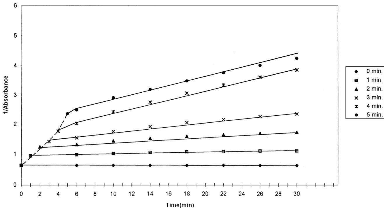
Fig. 5. Photolytic and photosensitized reactions of neutral red in cyclohexanone under anaerobic conditions.
