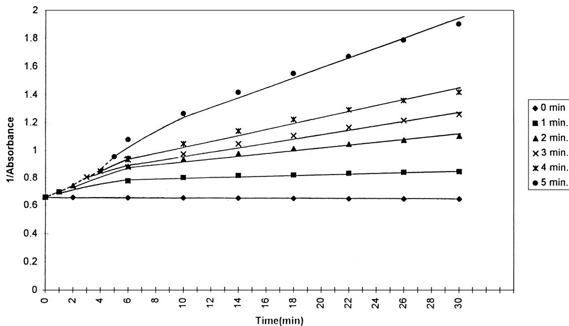
Fig. 3. Photolytic and photosensitised reactions of neutral red in cyclohexanone under aerobic conditions.
